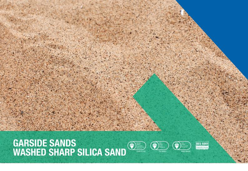
A washed sharp sand conforming to BS EN 12620, 13043, 13139.
